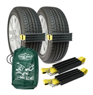
These things are made from EPDM Rubber with a webbed strap and D-Ring buckle, that you strap to your wheel. You then slowly power yourself out of the bog, the Tracgrabber providing something akin to a large tread block. Trac-Grabbers are an inventive designed block to help a slipping tyre to extract itself from a poor traction situations.
