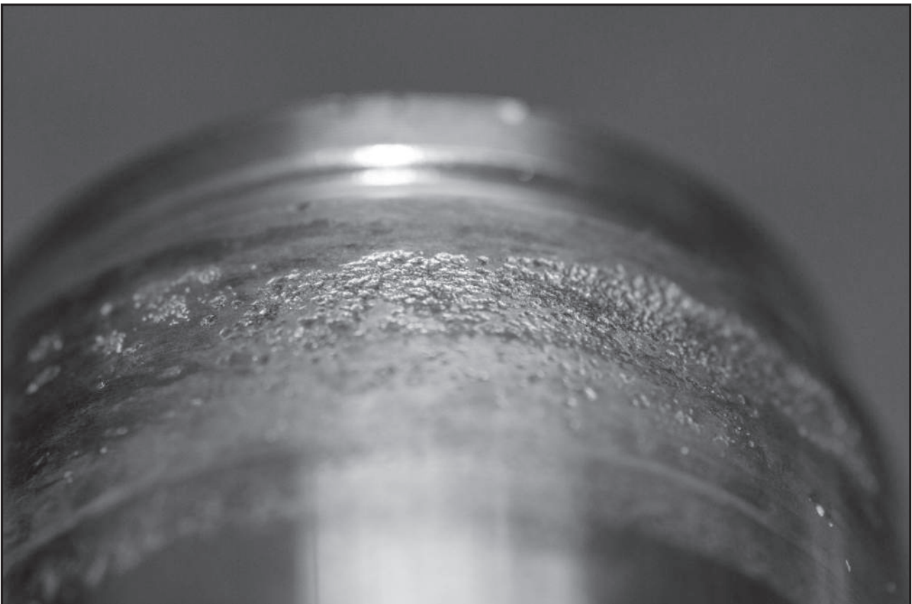
Pitting on the brake piston
