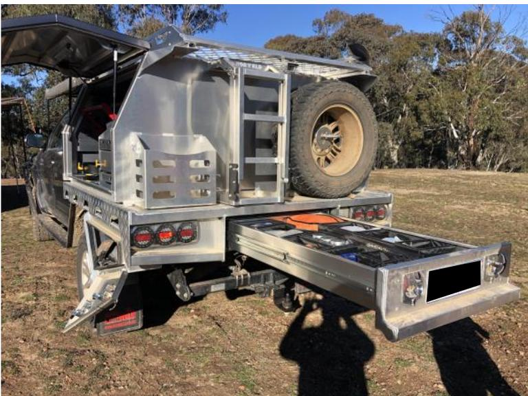
A trundle tray at the back is used to hold recovery gear, tools, spares, and other bits and bobs. Mike and Keryn found some fabric boxes from IKEA that fit perfectly and neatly arrange everything into easy to see and access compartments.
