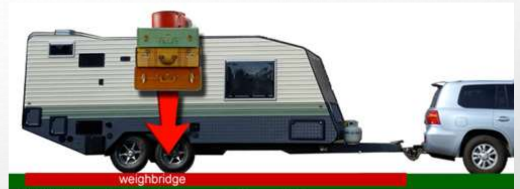
GTM Loaded and connected to vehicle.
